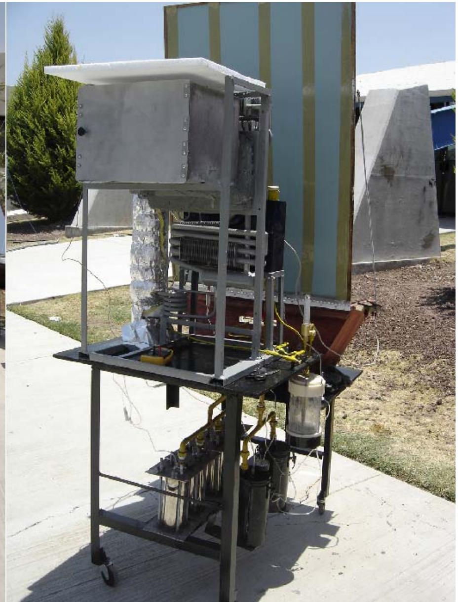
Tolokatsin 3 with solar refrigerator (photo to the right), and solar hot plate (photo to the left)
